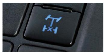
The Rear Differential Lock system helps secure traction when driving in muddy terrain, or in the unlikely situation when the vehicle is stuck. The vehicle is equipped with a solenoid switch differential lock system.
