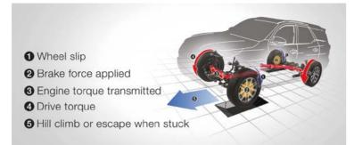
Active Traction Control (A-TRC)\*: When driving off-road or in slippery conditions, A-TRC applies brake pressure to prevent wheels from spinning during acceleration.
