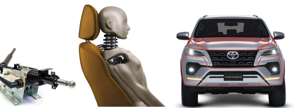
Collapsible Steering Column Breakaway and collapsible structures of the steering column help absorb impact energy.
