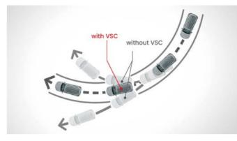
Vehicle Stability Control (VSC) to keep you in control and the vehicle pointing straight when on slippery surfaces by individually applying braking to each tyre where necessary.
