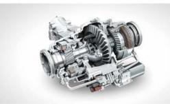
A Limited Slip Differential (LSD)\*\* that aims to ensure maximum available traction during wheel-spin situations by transmitting power to the tyre with the most grip. This will assist the driver in traversing mud and other soft surfaces; and provides better control during extreme cornering.
