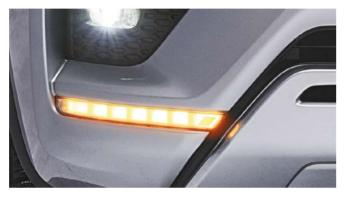
The angular headlamp design has been realised by separating the turn signal/position lamp from the headlamp.
