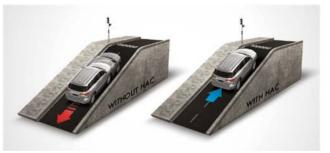
Hill-Assist Control (HAC), so that you don't need to worry about rolling back when pulling off from a sharp incline.
