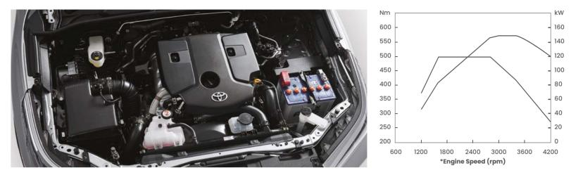
The New Generation 2.8-liter Diesel engine (IGD-FTV) has been optimally tuned for higher output and enhanced fuel economy. Refinements have been made to the Variable Nozzle Turbocharger and Intercooler, which contribute to both higher power and torque output with better fuel economy. The result - a prodigious +20kW Power output improvement and +50Nm Torque improvement from the previous generation engine.
